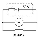
The reading of the voltmeter is 1.20 V.
