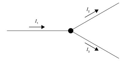
The currents in the three wires are related by  $I_1 = I_2 + I_3$ .
